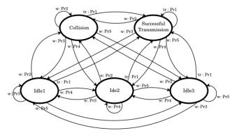
Fig. 1: MDP of collision handling at the wake-up plane Pr1= pr(successful transmission\s  $\in S$ , a=tr), Pr2= pr(collision\s  $\in S$ , a=tr), Pr3= pr(idle1\s  $\in S$ , a=w), Pr4= pr(idle2\s  $\in S$ , a=w), Pr5= pr(idle3\s  $\in S$ , a=w)
