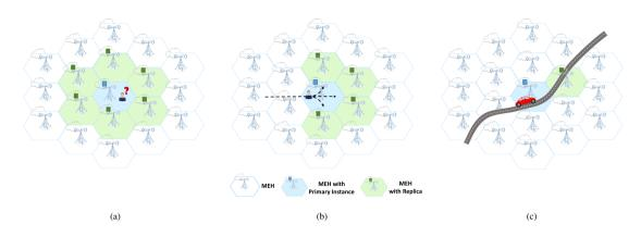
Figure 8. Examples of replicas deployment in a cellular network with naive approach (a), user direction prediction (b), and vehicular mobility prediction (c).
