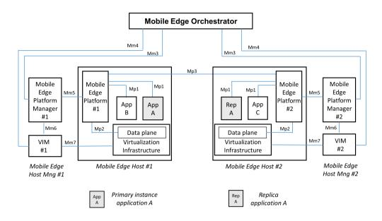
Figure 1. Architecture of the replication-based MEC framework.
