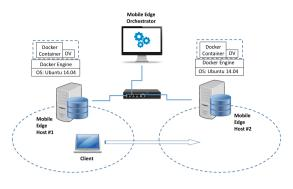
Figure 3. Setup testbed environment.
