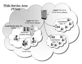
Fig. 1. A two-tiered network architecture: A number of local video servers are distributed in a wide service-area network. Popular video data are replicated at local servers to be locally served while the central server provides the whole area with unpopular items
