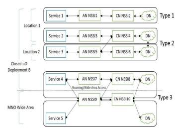
Fig 6. Deployment B: One closed network for multiple locations.
