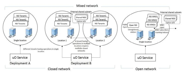
Fig 4. General overview of the of different micro-operator network deployments.
