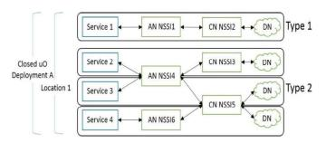
Fig 5. Deployment A: one closed network with both Type 1 and 2 NSI.
