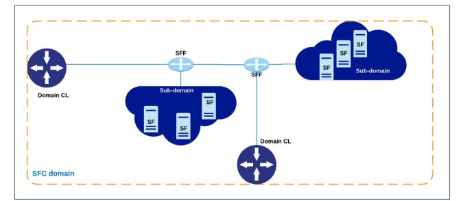
Figure 2: An example of Service Function Chaining Architecture, where the SFs in the sub-domain are visible to the SFC domain's SFFs.
