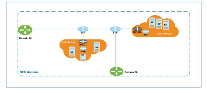
Figure 3: Architecture of Hierarchical SFC, where the SFC sub-domains are seen as single SFs to the higher SFC domain.
