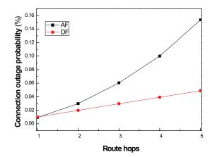
Fig. 2. Connection outage probability varies with the number of hops of a route under AF and DF schemes..
