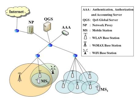
Fig. 2. Envisioned architecture for dynamic QoS negotiation in next-generation wireless networks.
