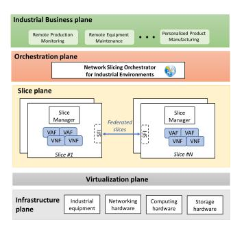
Fig. 2. Framework architecture for the orchestration of industrial network
