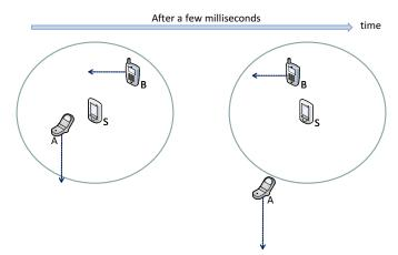
Fig. 2. A simple scenario that illustrates the inadequacy of the partner selection scheme based on only signal strength of the mobile nodes.
