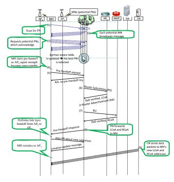
Fig. 1. Exchange of signaling messages in PHMIPv6 upon an inter-MAP handoff.
