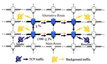
Fig. 2. A simplified simulation topology: a single TCP connection over the most congested area in the constellation (USA region).
