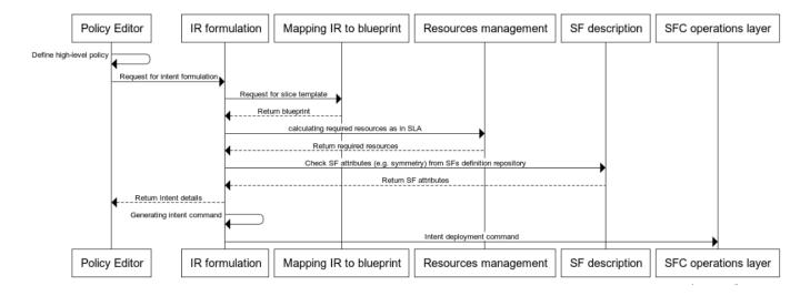
Fig. 3: Workflow for SFC intent deployment in the symmetry-aware SFC framework for 5G networks.
