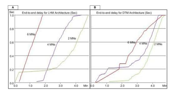
Figure 7: End-to-end delay results for LHM and DTM Architectures
