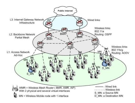
Figure 1: Wireless mesh network baseline architecture.
