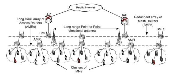
Figure 4: Long haul mesh architecture.
